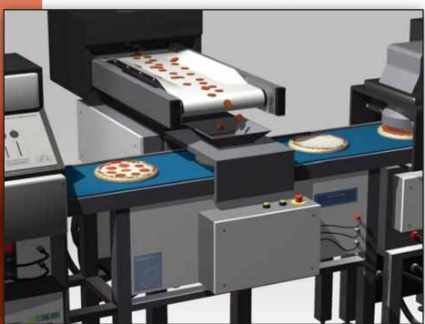
CenterClean belts are constructed with flexible urethane and sealed Kevlar® tension members. This construction allows CenterClean belts to be troughed and run on small diameter pulleys with minimal belt stretch.
