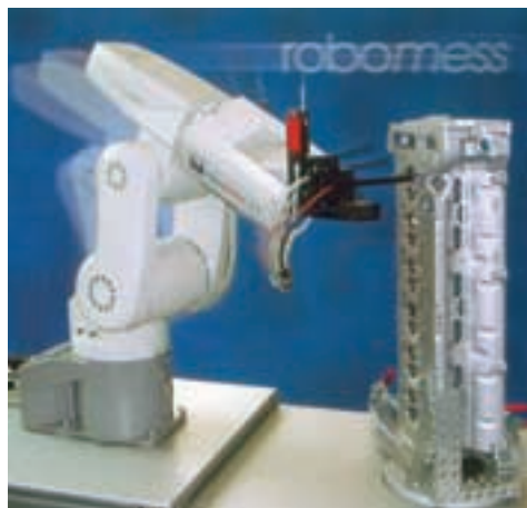
Multisensor measuring robot in a car engine factory of a famous motor car manufacturer, using the DIAVITE roughness meter
